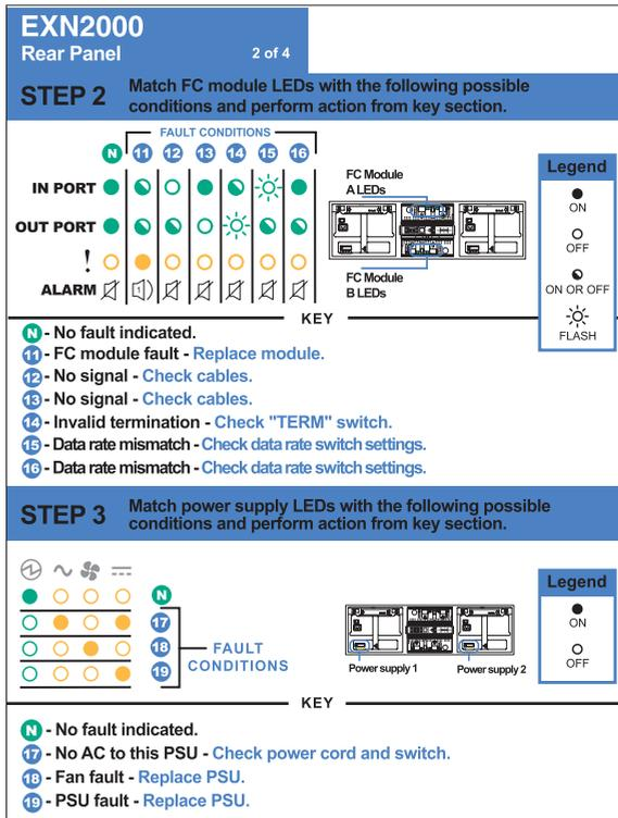
Figure 7. EXN2000 rear panel quick reference card
