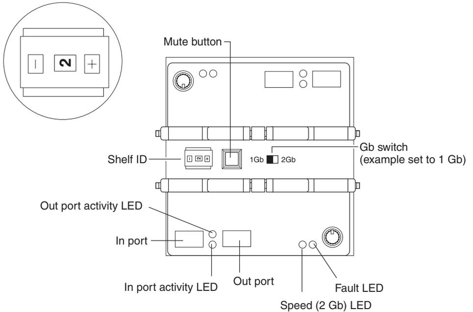
Figure 6. Location of the LEDs for an ESH2
